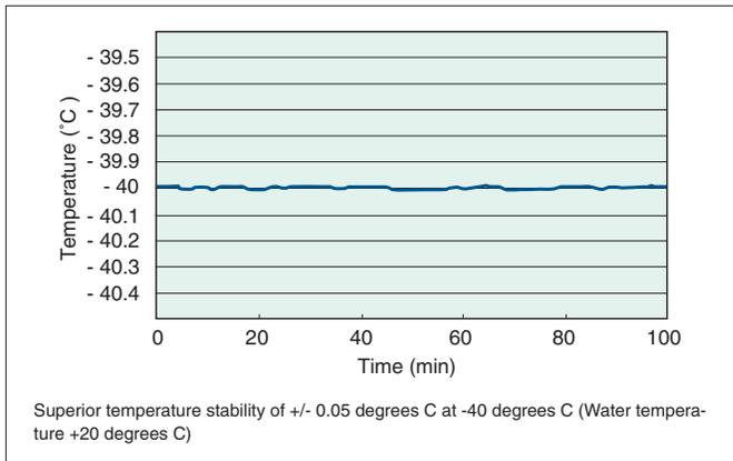
Fig. 7 Temperature stability
