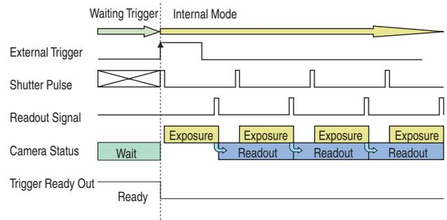
Fig. 14 Start trigger (positive edge)
