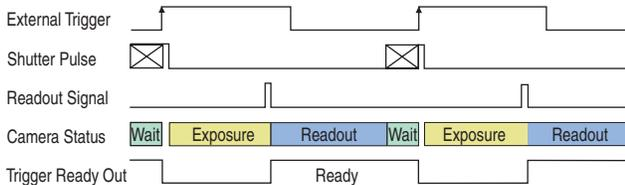
Fig. 16 Trigger ready out
