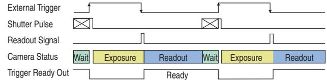
Fig. 12 Level trigger (positive edge)
