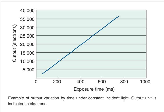
Fig. 10 Linearity in high dynamic range mode
