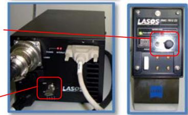
The laser ventilation keeps turning for 4-5min. **Don't switch the MAIN SWITCH yet.**
