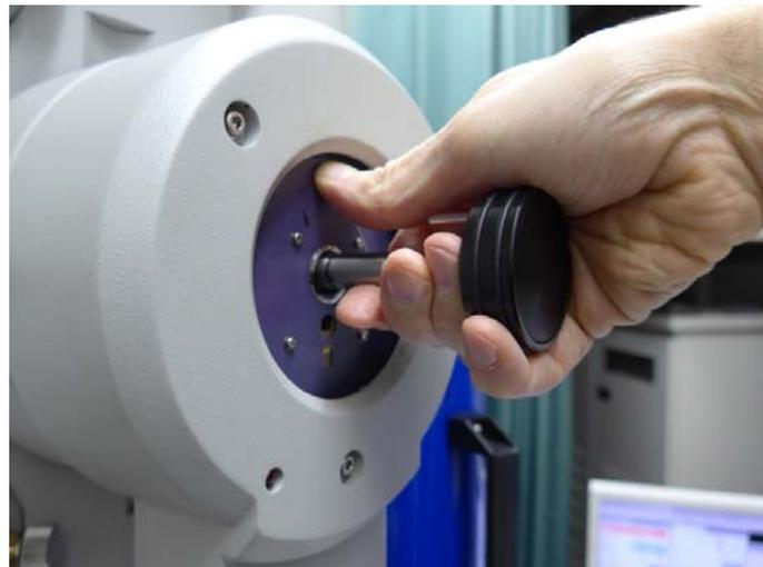
4. Position the specimen holder in its outside stand use the needle to lift the grid-holding ring. Put
