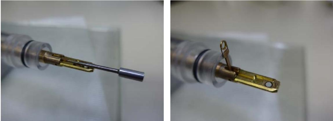
grid onto the opening of the holder, position it exactly and close the ring. Never touch the holder tip with your hands.
